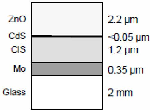
Fig. 2 A general schematic diagram of the AZO/  $\text{CuInSe}_2$  solar cell [Source : ARCO Solar] . A ZnO thickness of 2.2  $\mu\text{m}$  was much thicker than conventional TCO films for the same light transmission .
